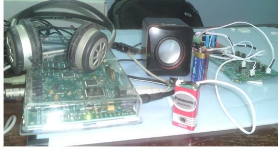
Figure 9: Experimental setup of the ANC system hardware.
