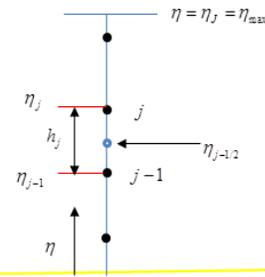
Fig. 2. Typical grid structure for difference approximations
