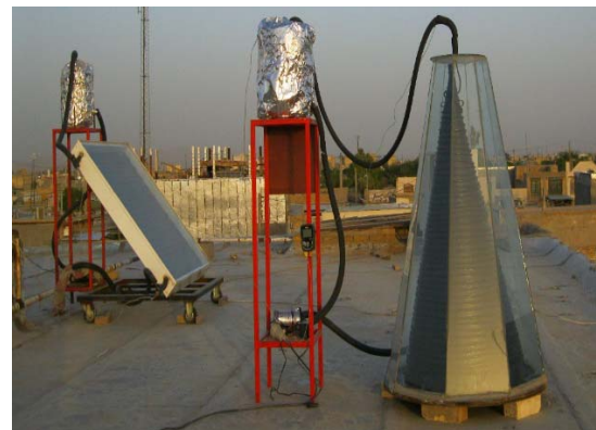
Fig. 3. The conical solar collector in setup
