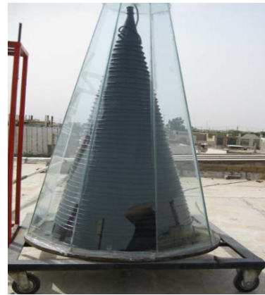
Fig. 2. Piping and covering install on conical solar collector
