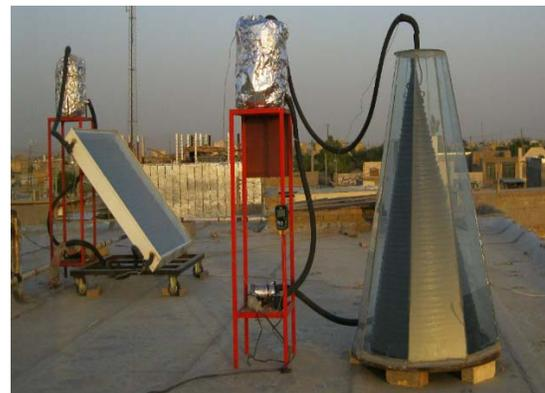
Fig. 3. The conical solar collector in setup
