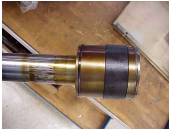
Fig. 1. Varnish formation on Inlet Guide Vane (IGV) valve from a gas turbine (Courtesy of Clarus technologies)
