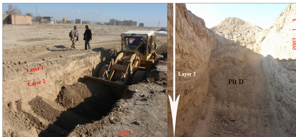
Figure 8: Mafin Abad: The stratigraphy of Pit D. The second layer consists of dense clay sediments with a thickness of 3.5 m
