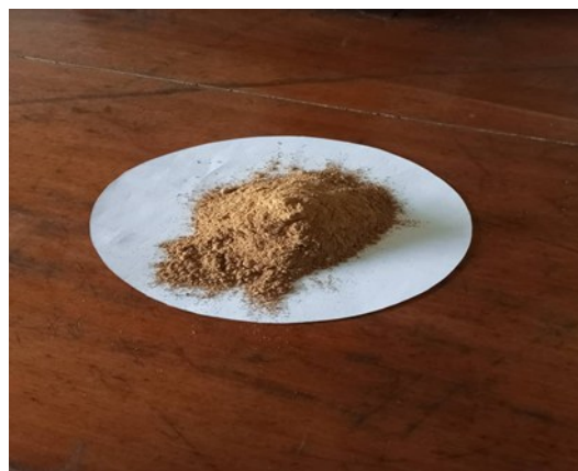
Fig. 2b. Milled sample of Azara Barite.
