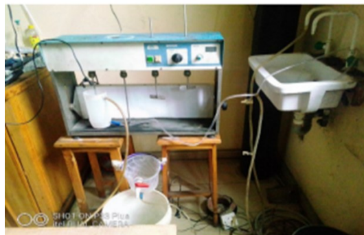
Fig. 3. Experimental setup for desliming the Azara Barite sample.
