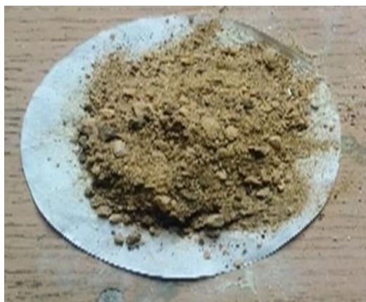
Fig. 2a. Crushed sample of Azara Barite.
