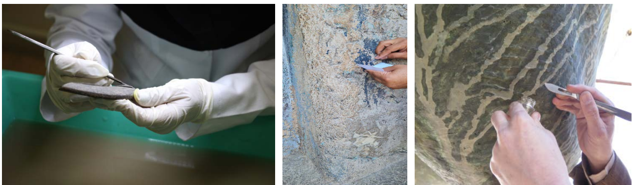
Figure. 1: Types of Purpose-based Sampling: Left) Sampling residues from historical pottery to investigate the usage of the artefact; Middle) Sampling sediments and corrosion from the bronze statue of Nader Shah Afshar in Mashhad to identify and analyse corrosion mechanisms; Right) Non-destructive sampling from the surface of the Persepolis stone plinths to identify biological contaminants.
