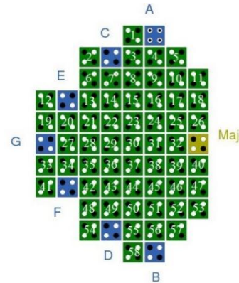
Fig.13.The proposed fault-tolerant 7-input Majority Gate (numbered cells)
