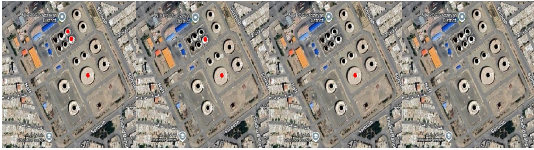
Fig B.1. Geographical map of the Sabzevar region showing simulation stages from the initial scenario (Tank 13 ignition) to domino process completion, with color-coded tank status (blue: normal, yellow: heated, red: ignited, black: extinguished)
