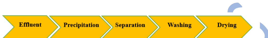
Fig. 2. Overall stages of the desalination brine management process
