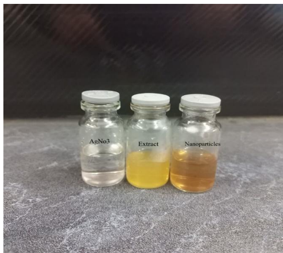
Fig. 1. Visual observation of color change during the green synthesis of silver nanoparticles using ethanolic saffron extract: (left) colorless \text{AgNO}_3 solution, (middle) light yellow saffron extract, and (right) yellowish-brown solution indicating the formation of silver nanoparticles due to SPR.
