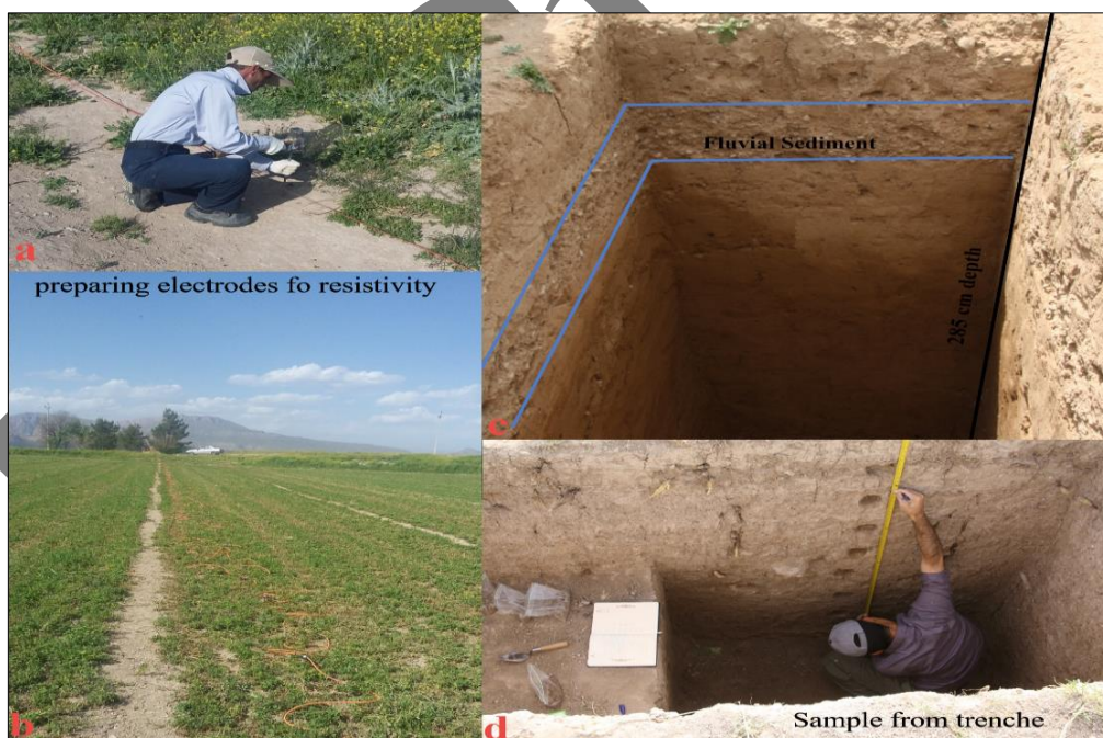
Figure 6: a, b: preparing electrodes for geoelectrical study (depth of the geoelectrical study is 20m) – c: Sample collection was based on sedimentary layer changes, d: Sampling was conducted based on regular intervals. (After:10/06/2022).
