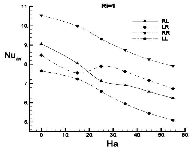
**Fig. 6.** Variations of average Nusselt number with Hartmann number at four different configurations ( $\xi=0.06$ ).
