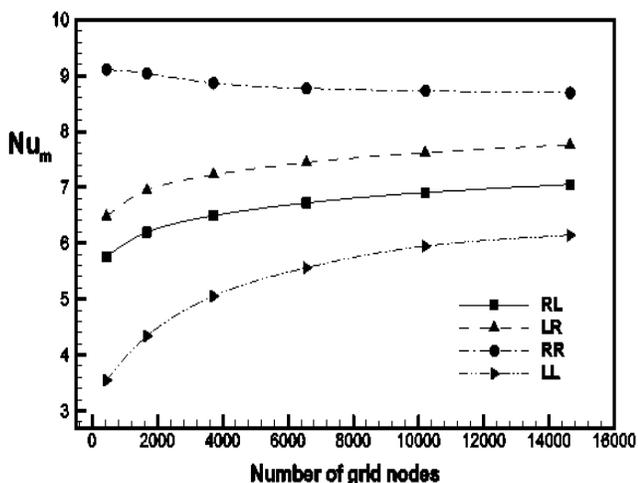
Fig. 3. Grid independency study: average Nusselt number at different grid densities.
