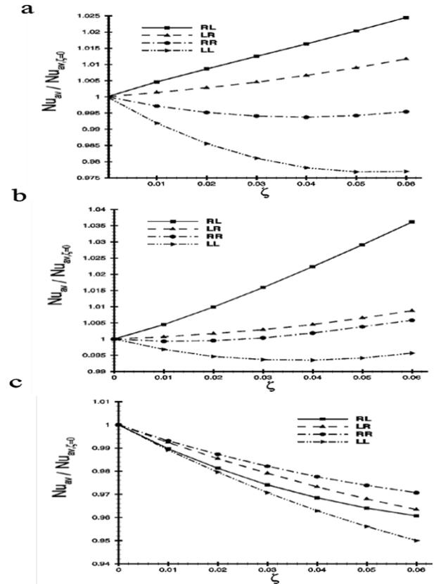
Fig. 7. Variations of the average Nusselt number ratio at hot wall with solid volume fraction at  $Ha=35$  for different configurations a)  $Ri=0.1$ , b)  $Ri=1$ , c)  $Ri=10$ .
