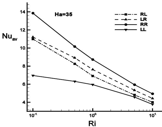
**Fig. 5.** Variations of average Nusselt number with Richardson number at four different configurations ( $\xi=0.06$ ).
