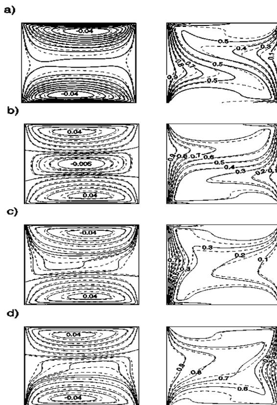
Fig. 4. Streamlines (on the left) and isotherms (on the right) for Cu-water nanofluid with  $\xi=0.06$  (solid line) and pure fluid (dashed line) a) RL, b) LR, c) RR and d) LL configuration ( $Ri=1$ ,  $Ha=35$ ).
