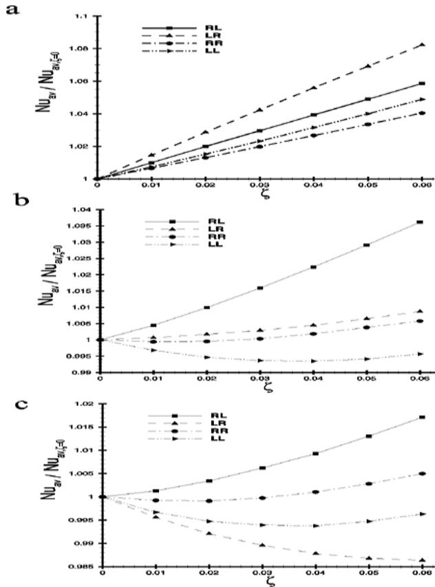
**Fig. 8.** Variations of the average Nusselt number ratio at hot wall with solid volume fraction at  $Ri=1$  for different configurations a)  $Ha=0$ , b)  $Ha=35$ , c)  $Ha=55$ .
