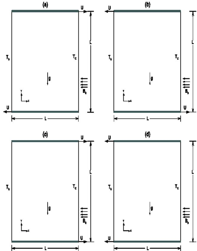
**Fig. 1.** Schematic flow configuration of the problem: a) RL Configuration, b) LR Configuration, c) RR Configuration and d) LL Configuration.
