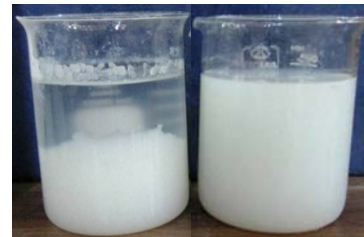
Fig.1. a) Propylene glycol mixed with ZnO (b) propylene glycol nanofluid after sonication.
