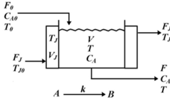
FIGURE 5. Continuous Stirring Tank Reactor
