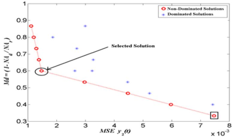
FIGURE 10. Feasible Pareto-front for Two Objectives, x-axis: is the MSE of the Second Output, y-axis: Objective Value Related to Don't Cares, when  $N_R = 1$ . Selected Solution has been Highlighted
