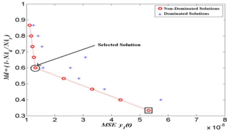
FIGURE 9. Feasible Pareto-front for Two Objectives, x-axis: is the MSE of the First Output, y-axis: Objective Value Related to Don't Cares, when  $N_R = 1$ . Selected Solution has been Highlighted
