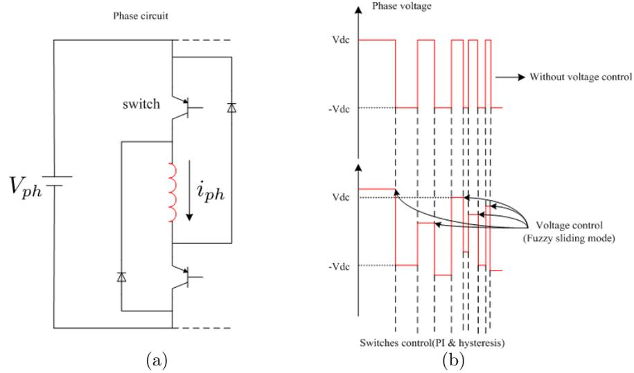
FIGURE 6. (a) Motor Phase Circuit and (b) Control Procedure Schemes
