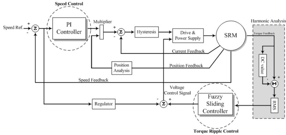
FIGURE 7. Block Diagram of SRM Drive with the Proposed Structure
