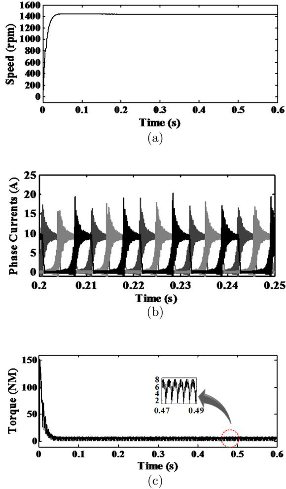
FIGURE 8. (a) Motor Speed, (b) Phase Currents and (c) Motor Torque without Torque Ripple Control
