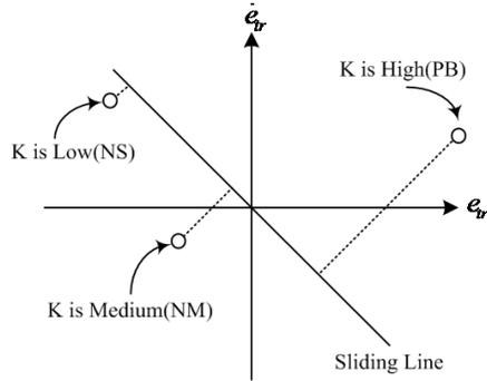
FIGURE 4. Determination of K Using Fuzzy Sets
