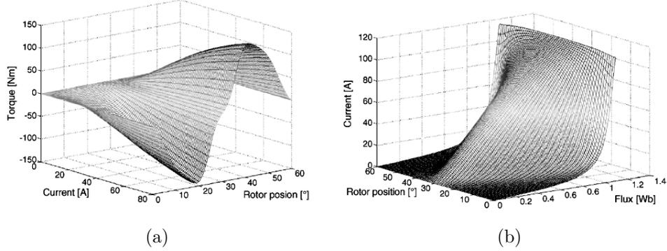
FIGURE 1. Lookup Table of (a) Torque-current-position and (b) Flux-current-position
