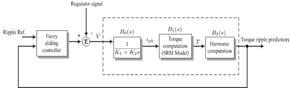
FIGURE 2. Block Diagram of the Torque Ripple Reduction Loop
