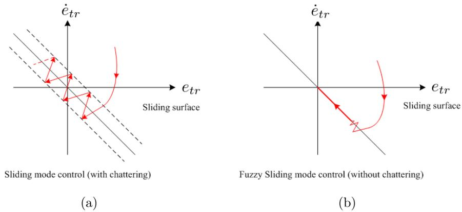
FIGURE 5. Trajectory of the Sliding State (a) without Using Fuzzy Method and (b) with Fuzzy Method
