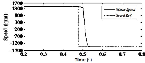
FIGURE 10. Response of Speed Reversal in the SRM
