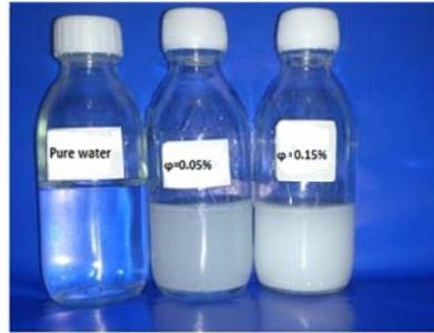
Fig.2. Stability photograph of  $\gamma\text{-Al}_2\text{O}_3$  nanofluids after 24 h
