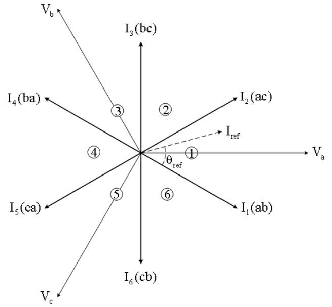
FIG. 4. Space vectors of the input current.
