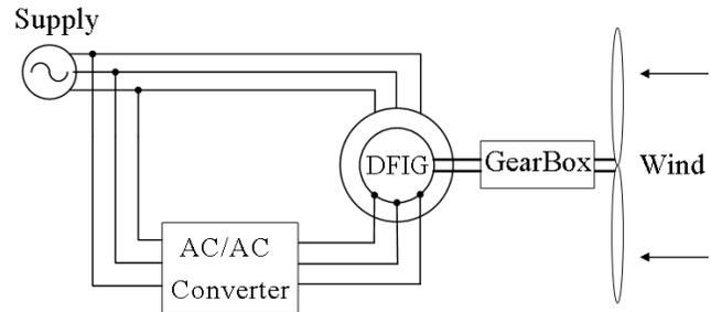
FIG. 1. Wind turbine based on the DFIG.
