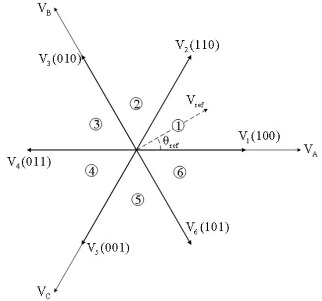
FIG. 5. Space vectors of the output voltage.
