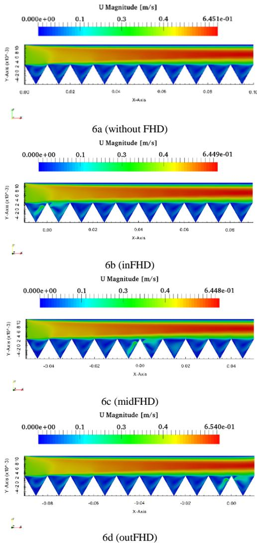
**Fig. 6.** Velocity contour comparison in  $q'' = 530 \text{ W/m}^2$
