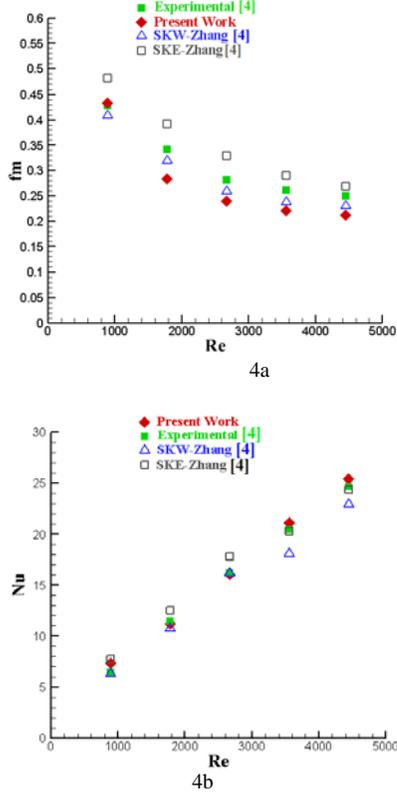
Fig. 4. Validation; a) average Nusselt number b) friction coefficient
