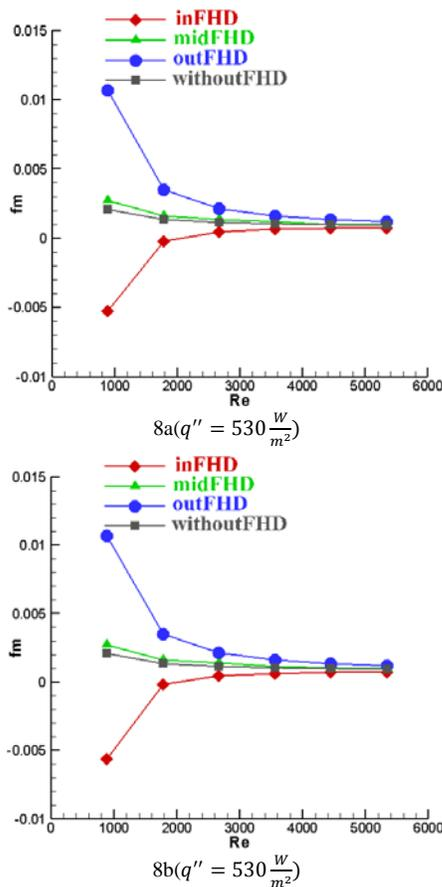
Fig. 8. Average friction factor in respect to Reynolds number
