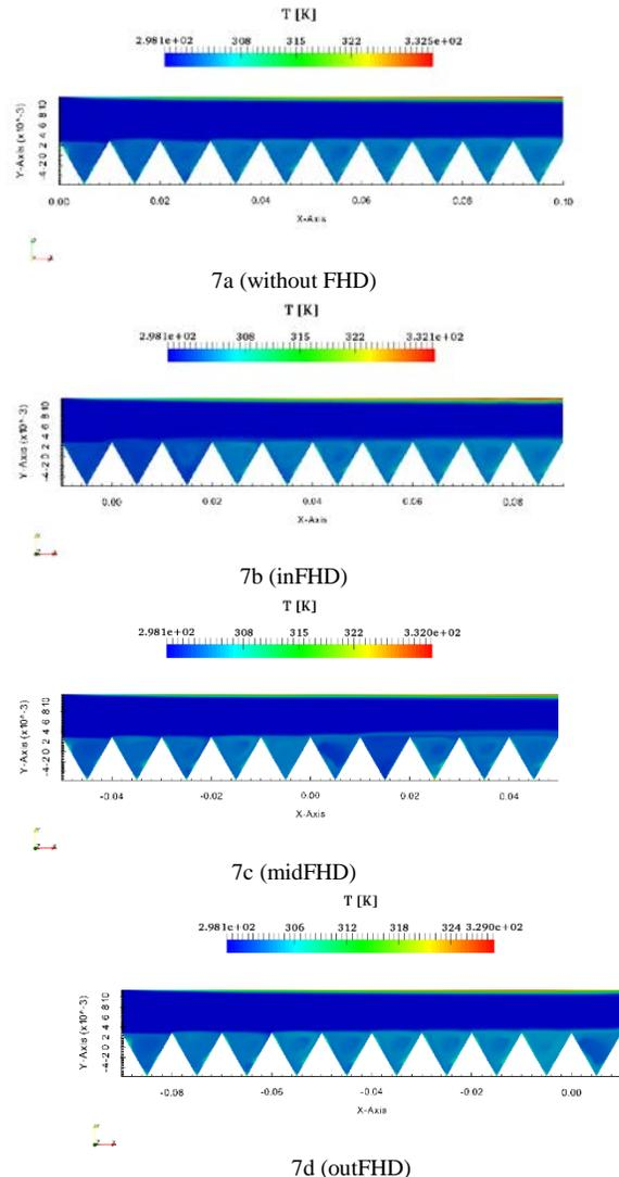
**Fig. 7.** Temperature contour comparison in  $q'' = 530 \text{ W/m}^2$
