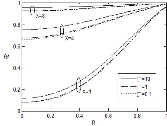
Fig. 8. Effect of the Forchheimer number on the distribution of the fluid temperature at different sections through the micro-tube ( $Kn = 0.01, Pe = 100, Da = 1, Bi = 1, K_R = 1$ )
