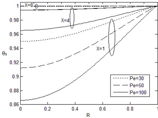
**Fig. 12.** Effect of the Peclet number on the distribution of the solid temperature at different sections through the micro-tube ( $Kn = 0.01, Da = 1, \Gamma = 10, Bi = 1, K_R = 1$ )
