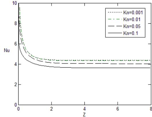
**Fig. 13.** Effect of the Knudsen number on the distribution of the local Nusselt number through the micro-tube ( $Pe = 100, Da = 1, \Gamma = 10, Bi = 1, K_R = 1$ )
