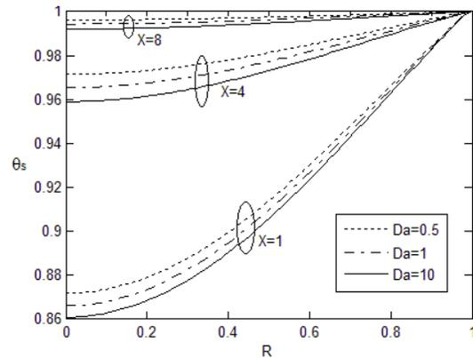
Fig. 9. Effect of the Darcy number on the distribution of the solid temperature at different sections through the micro-tube ( $Kn = 0.01, Pe = 100, \Gamma = 10, Bi = 1, K_R = 1$ )
