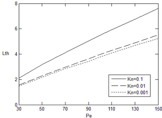
**Fig. 19.** Effect of the Peclet number on the thermal entry length ( $Kn = 0.1, \Gamma = 10, Da = 1, Bi = 1, K_R = 1$ )
