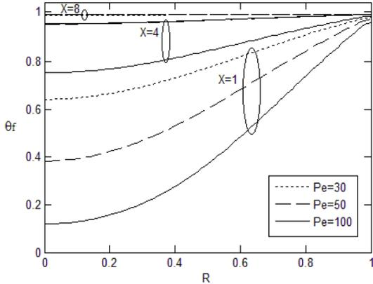
**Fig. 11.** Effect of the Peclet number on the distribution of the fluid temperature at different sections through the micro-tube ( $Kn = 0.01, Da = 1, \Gamma = 10, Bi = 1, K_R = 1$ )
