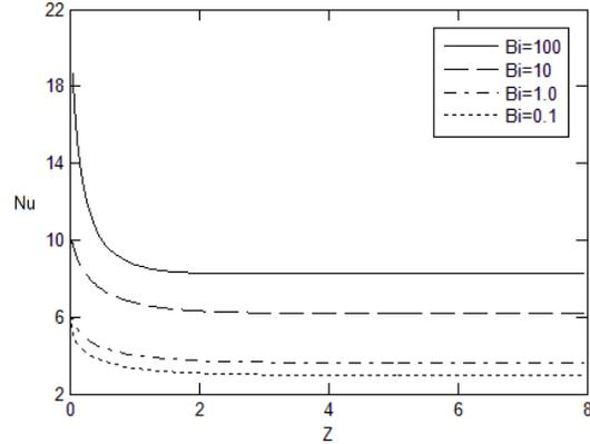
**Fig. 20.** Effect of the Biot number on the distribution of the local Nusselt number through the micro-tube ( $Kn = 0.1, Pe = 100, \Gamma = 10, Da = 1, K_R = 1$ )
