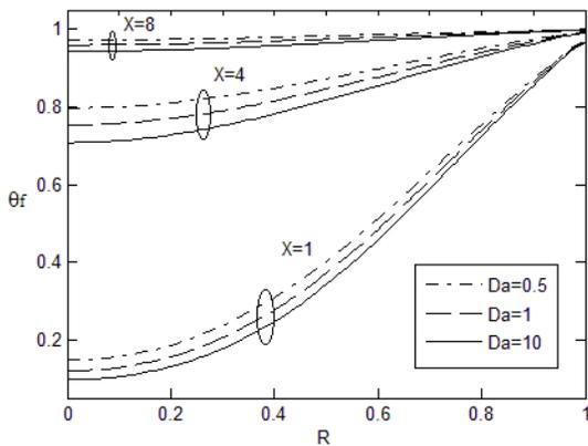
Fig. 7. Effect of the Darcy number on the distribution of the fluid temperature at different sections through the micro-tube ( $Kn = 0.01, Pe = 100, \Gamma = 10, Bi = 1, K_R = 1$ )
