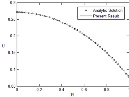
**Fig. 2.** The obtained velocity distribution compared with that of the exact solution of Haddad et al. [6] ( $Kn = 0.1, Da = 1, \Gamma = 0$ )
