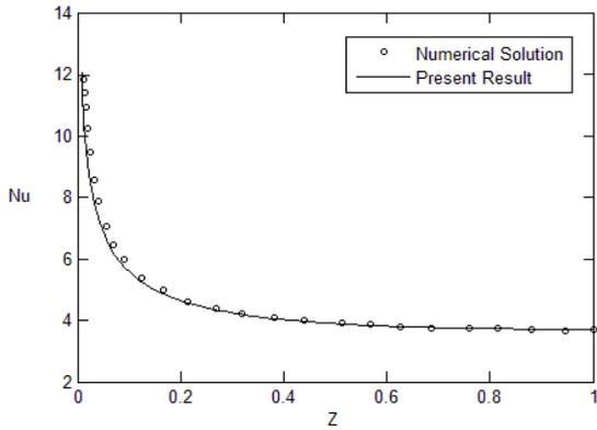
**Fig. 3.** The obtained distribution of the local Nusselt number compared with that of the numerical results of Haddad et al. [6] ( $Kn = 0.01, Pe = 35, Da = 1, \Gamma = 0.1$ )
