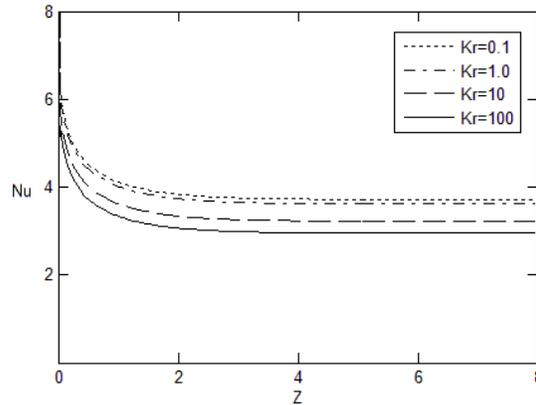
**Fig. 21.** Effect of the modified thermal conductivity ratio on the distribution of the local Nusselt number through the micro-tube ( $Kn = 0.1, Pe = 100, \Gamma = 10, Da = 1, Bi = 1$ )
