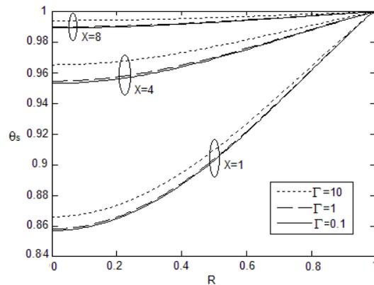
Fig. 10. Effect of the Forchheimer number on the distribution of the solid temperature at different sections through the micro-tube ( $Kn = 0.01, Pe = 100, Da = 1, Bi = 1, K_R = 1$ )
