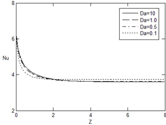
**Fig. 14.** Effect of the Darcy number on the distribution of the local Nusselt number through the micro-tube ( $Kn = 0.1, Pe = 100, \Gamma = 10, Bi = 1, K_R = 1$ )
