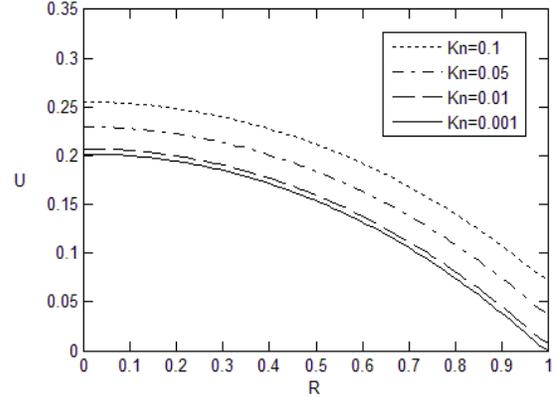
**Fig. 4.** Effect of the Knudsen number on the distribution of velocity ( $Da = 1, \Gamma = 1$ )
