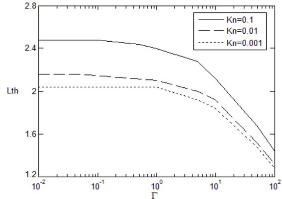
**Fig. 17.** Effect of the Forchheimer number on the thermal entry length ( $Pe = 100, Da = 1, Bi = 1, K_R = 1$ )
