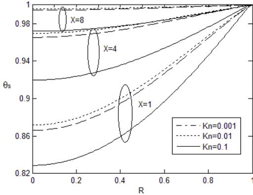
Fig. 6. Effect of the Knudsen number on the distribution of the solid temperature at different sections through the micro-tube ( $Pe = 100, Da = 1, \Gamma = 10, Bi = 1, K_R = 1$ )
