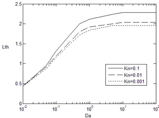
**Fig. 15.** Effect of the Darcy number on the thermal entry length ( $Pe = 100, \Gamma = 10, Bi = 1, K_R = 1$ )
