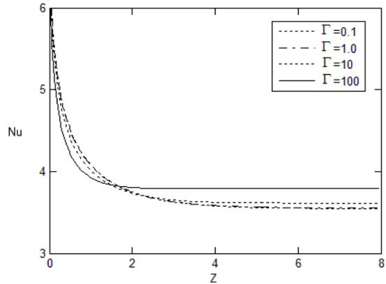
**Fig. 16.** Effect of the Forchheimer number on the distribution of the local Nusselt number through the micro-tube ( $Kn = 0.1, Pe = 100, Da = 1, Bi = 1, K_R = 1$ )
