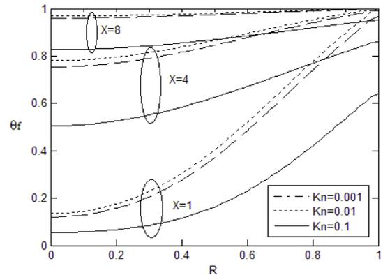
**Fig. 5.** Effect of the Knudsen number on the distribution of the fluid temperature at different sections through the micro-tube ( $Pe = 100, Da = 1, \Gamma = 10, Bi = 1, K_R = 1$ )
