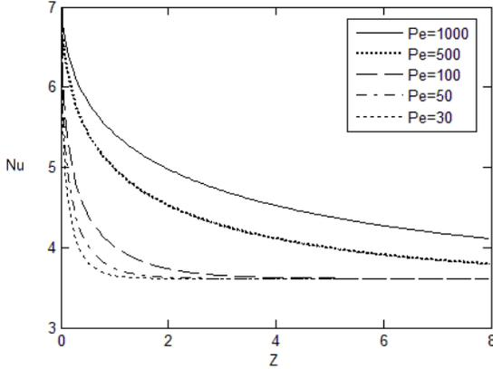
**Fig. 18.** Effect of the Peclet number on the distribution of the local Nusselt number through the micro-tube ( $Kn = 0.1, \Gamma = 10, Da = 1, Bi = 1, K_R = 1$ )
