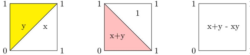
FIGURE 2. Linear Extensions of the Boolean Disjunction: Zadeh's Disjunction (left); Lukasiewicz's Disjunction (Middle); Probabilistic Sum (Right)
