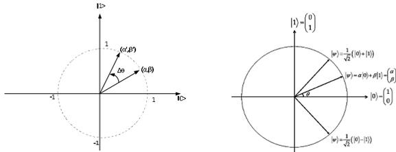
Fig.2. Polar plot of the rotation gate for Q-bit individuals [26] (left) and Hadamard gate (right)[32].
