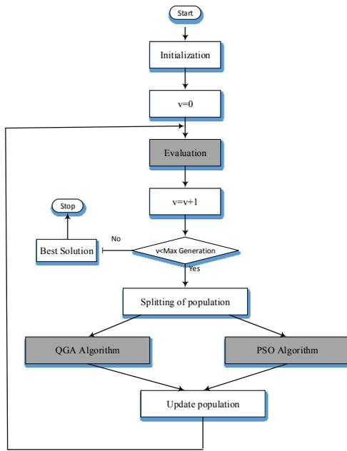
Fig. 5. Flowchart of QGA-PSO algorithm
