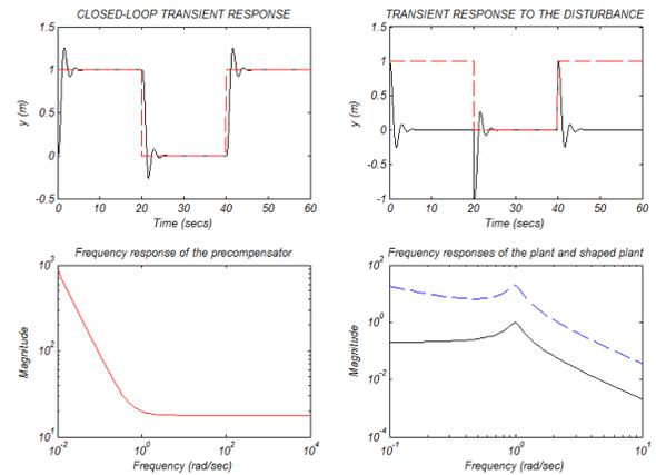
Fig.6.( Continued) Closed –open loop behavior of the system.
