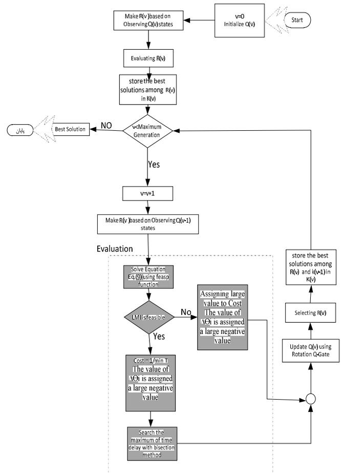
Fig. 4. Flowchart of QGA-LMI algorithm
