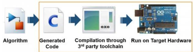
Fig. 11. Code generation procedure in MATLAB
