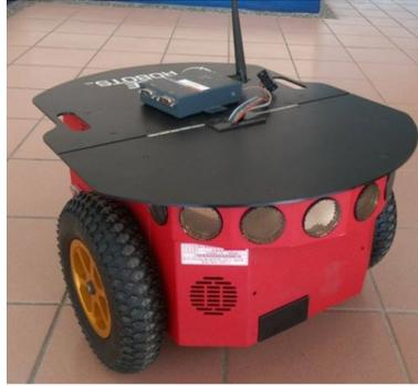
Figure 1: Pioneer 3-DX Mobile Robot.
