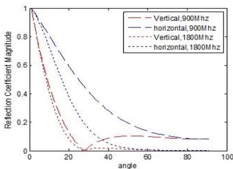
Fig. 2 The magnitudes of the reflection coefficients for a dry ground's surface with 4 cm SD of roughness [29].
