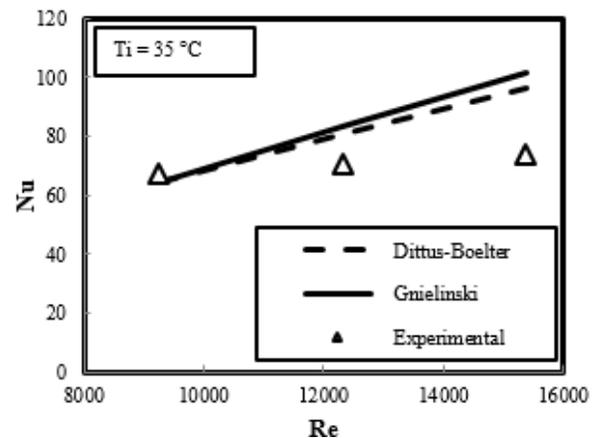
Fig. 3. Validation of experimental setup.
