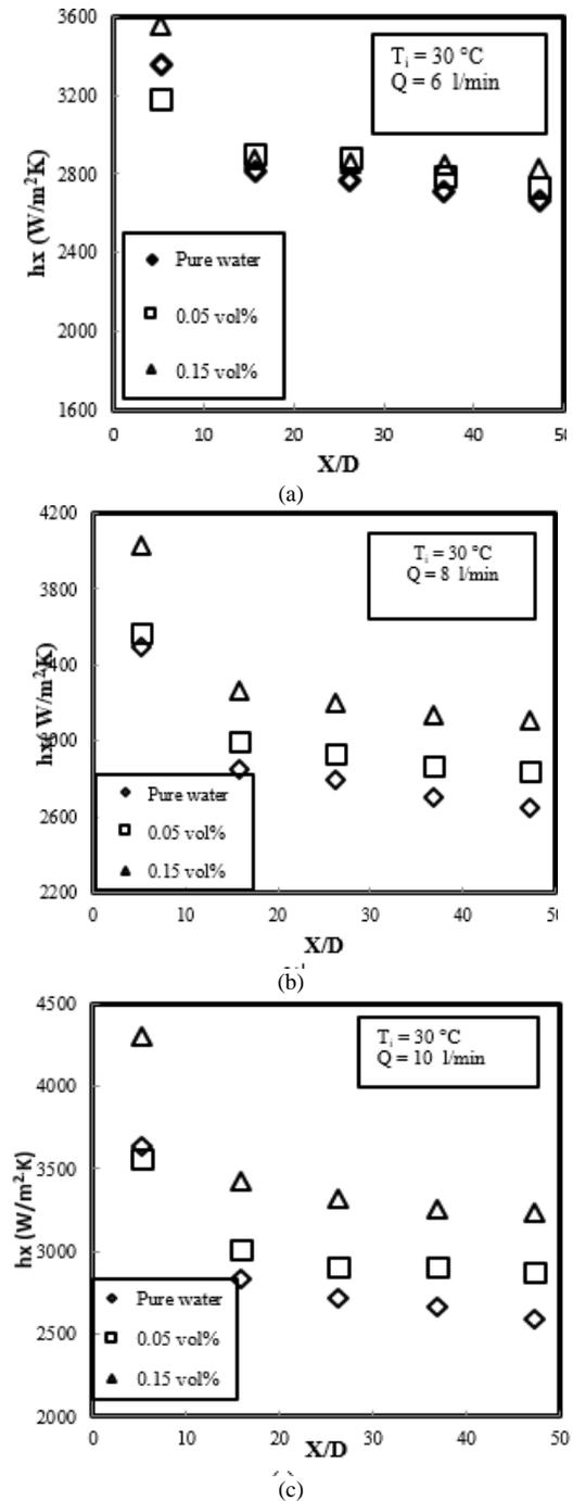
**Fig. 5.** Local heat transfer coefficient variation of MgO/water nanofluid along axial distance at  $T_i = 30$  °C, a)  $Q = 6$  l/min, b)  $Q = 8$  l/min, c)  $Q = 10$  l/min
