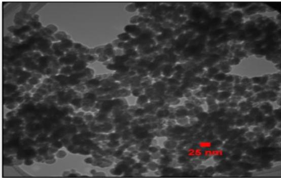
**Fig. 1.** TEM image of MgO nanoparticles
