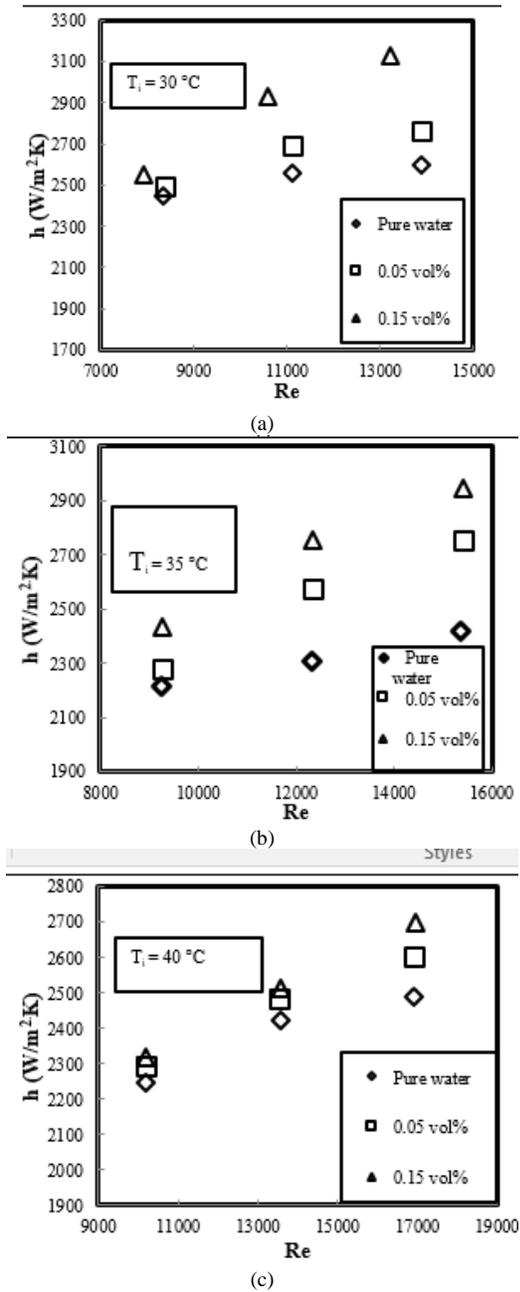
**Fig. 4.** Variation of average heat transfer coefficient of nanofluid with Reynolds number at the inlet temperatures of a) 30 °C, b) 35 °C, and c) 40 °C
