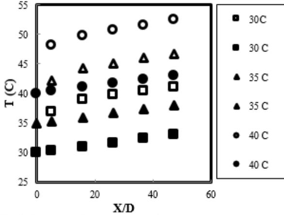
**Fig. 6.** Bulk and wall temperature profiles versus the dimensionless axial length, for three inlet temperatures include 30,35 and 40 °C, MgO-water nanofluid at 0.15 vol.% concentration and flow rate of 6 l/min and Nominal heat flux 4.5 kW/m<sup>2</sup>. (■,●,▲) Bulk and (□,○,△) wall temperatures.
