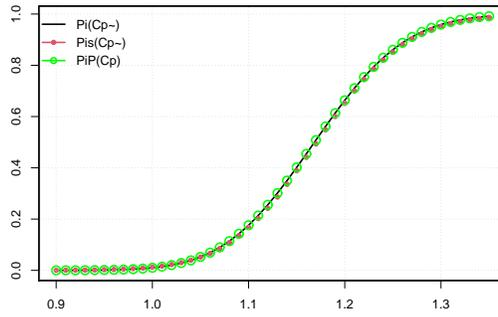
Figure 7: Plots of the power functions of three quality tests involves  $\Pi(C_{\bar{p}})$ ,  $\Pi_s(C_{\bar{p}})$  and  $\Pi_P(C_p)$  for the computed critical values based on the given values of  $\alpha = 0.01$ ,  $c_0 = 1.00$ , and the sample size  $n = 125$ .
