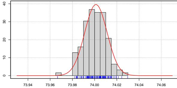
Figure 4: Kernel density estimation and histogram plot for 125 observed inside diameters.
