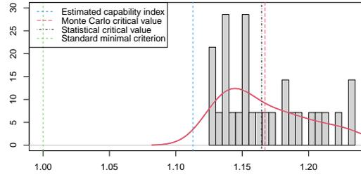
Figure 6: Histogram of simulated critical values in iterations of the Monte Carlo FQT with its kernel density estimation based on the specified linear fuzzy SLs.
