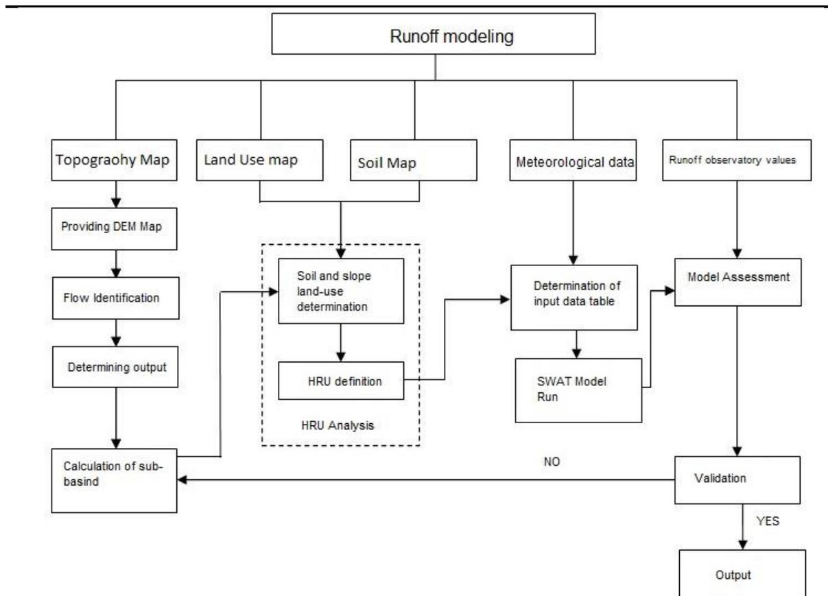
Fig 2. The runoff calculation flow chart with the help of hydrologic SWAT
