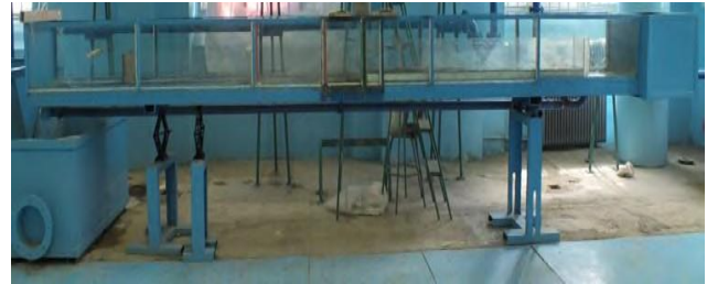
Fig.2. The flume used for the idealized dam-break experiments
