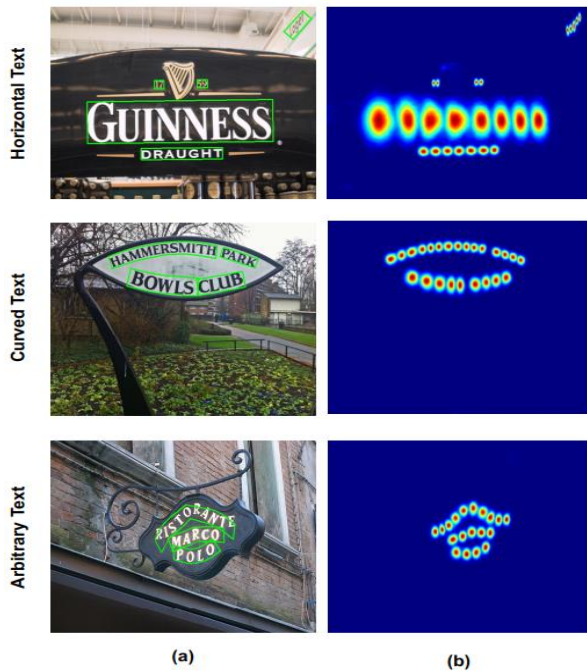
Fig. 1. The capability of the text detection results in any shape in CRAFT. (a) The polygon bounding box of the detected characters, (b) Gaussian heat-map of individual characters of the text.
