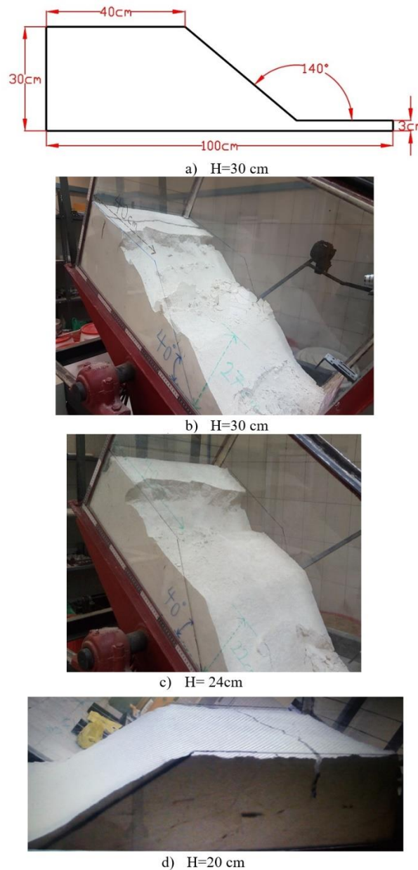
Figure 2- a) Schematic model with H=30cm, b) failed model in different heights.
