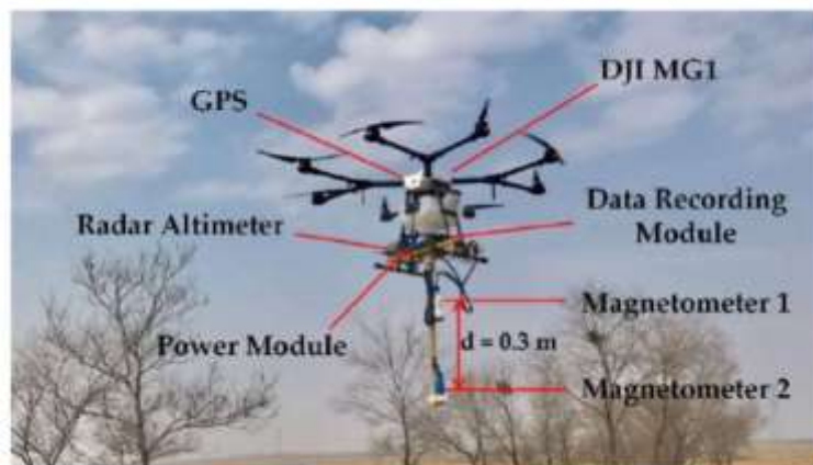
Figure 3. The Unmanned Aerial Vehicle (UAV)-magnetometer system, carrying two magnetometers, radar altimeter, GPS, data recording and power module. The top magnetic sensor is labelled as magnetometer 1 and the bottom magnetic sensor is labelled as magnetometer 2 [18].
