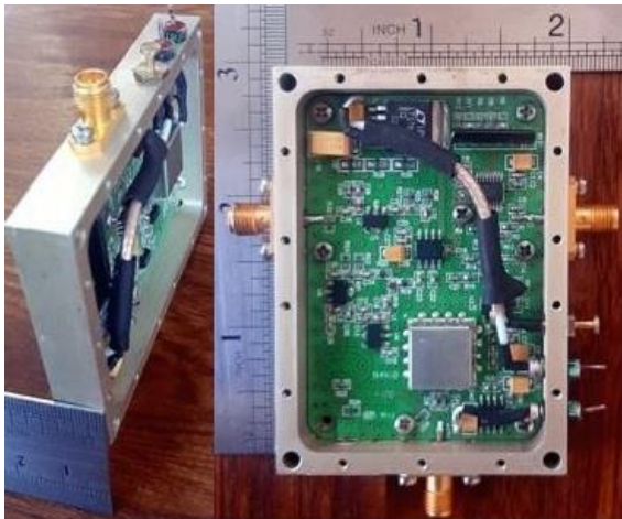
Fig. 12. The dimensions of module PLL implemented.
