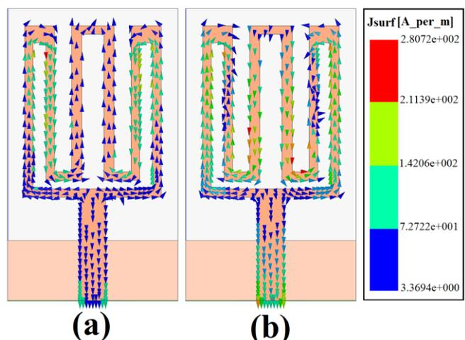
**Fig.5** Simulated surface current distributions on radiating patch for the proposed antenna (a) at 3.8 GHz and (b) at 5.5 GHz
