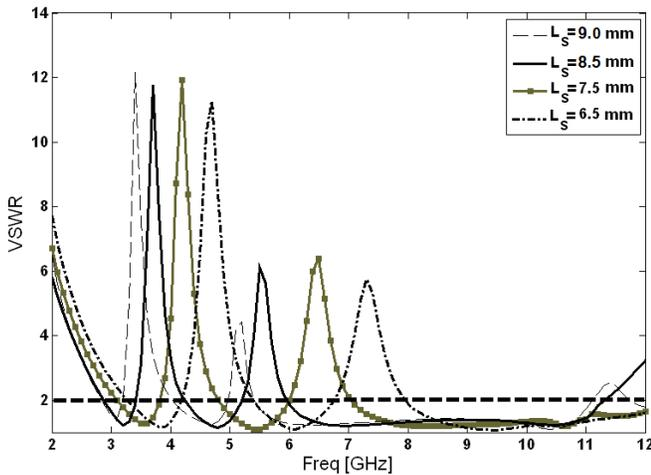
**Fig. 6.** Simulated VSWR characteristics for the proposed antenna with different values of  $L_s$ .
